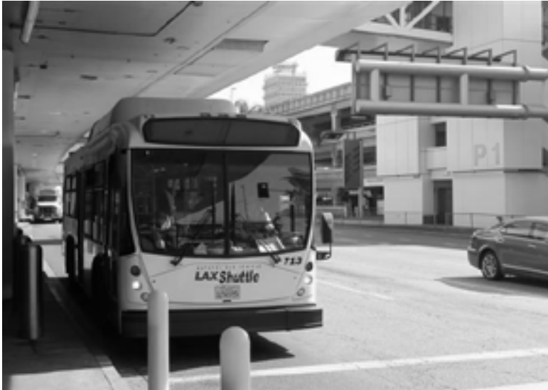
Shuttle buses at LAX run on compressed natural gas (photo courtesy of lawa.org).
